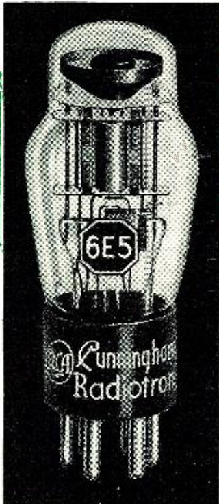
The FM tuning indicators shown here include the 6E5 and the 6AL7 tuning eye tubes along with a space-saving, side-indicating type tuning meter.
